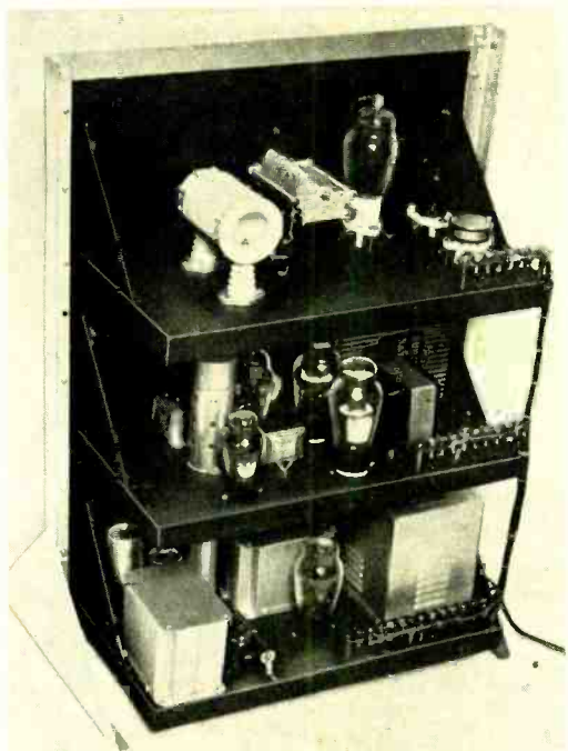
The transmitter is entirely contained in these three chassis in the homemade rack.
