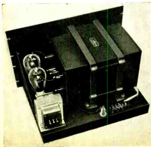
The heavy duty, high voltage power transformer and the rectifiers are mounted on this deck, at the left.
